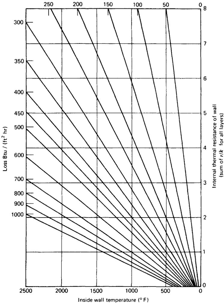
Fig. 45.8 Furnace wall losses as a function of composite thermal resistance.<sup>1</sup>
