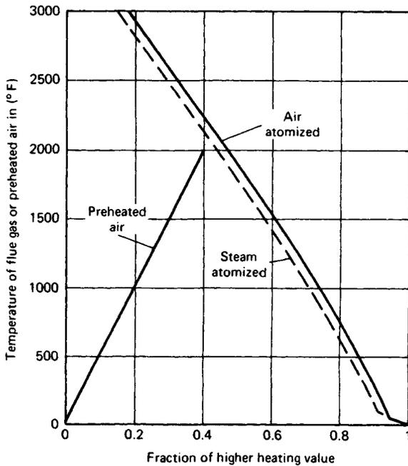
**Fig. 45.2** Available heat ratios for fuel oils with air or steam atomization.<sup>1</sup>
