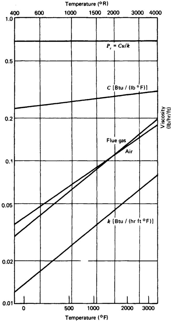
Fig. 45.9 Thermodynamic properties of air and flue gas.<sup>1</sup>
