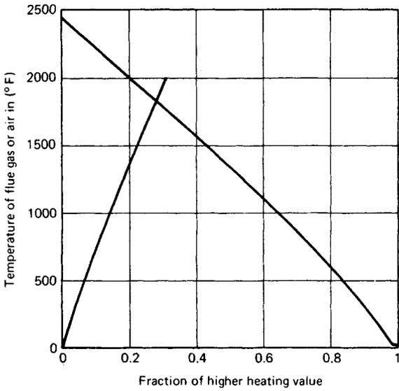
Fig. 45.4 Available heat ratios for blast furnace gas.<sup>1</sup>
