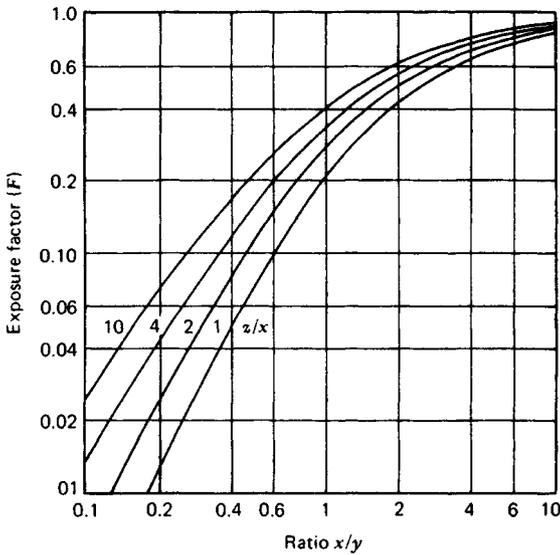
**Fig. 45.15** Radiation view factors for parallel planes.<sup>1</sup>
