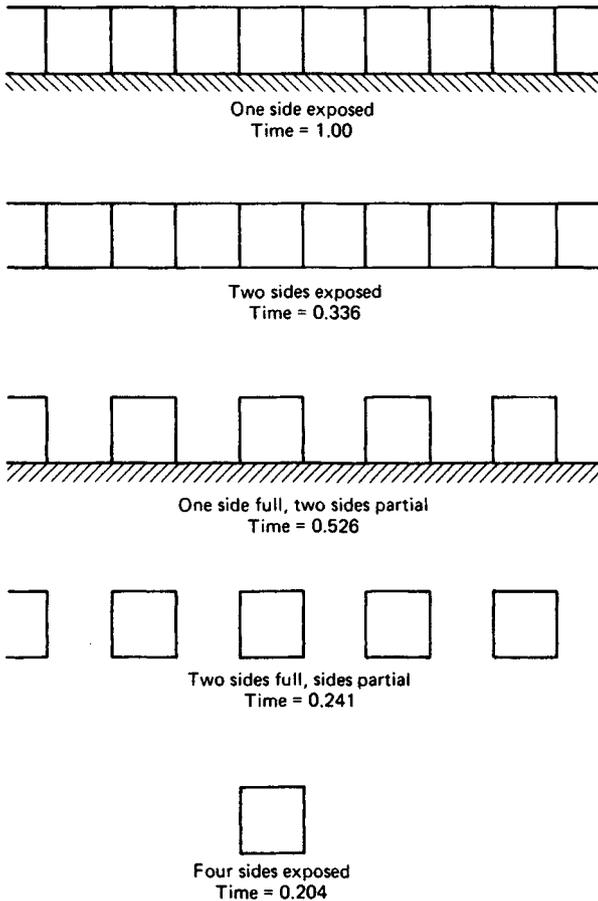
**Fig. 45.26** Heating time for carbon steel slabs to final surface temperature of 2300°F, as a function of thickness and final load temperature differential.<sup>1</sup>
