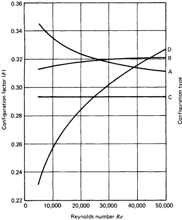
Fig. 45.30 Configuration factors for convection heat transfer, air or flue gas through tube banks.<sup>1</sup>
