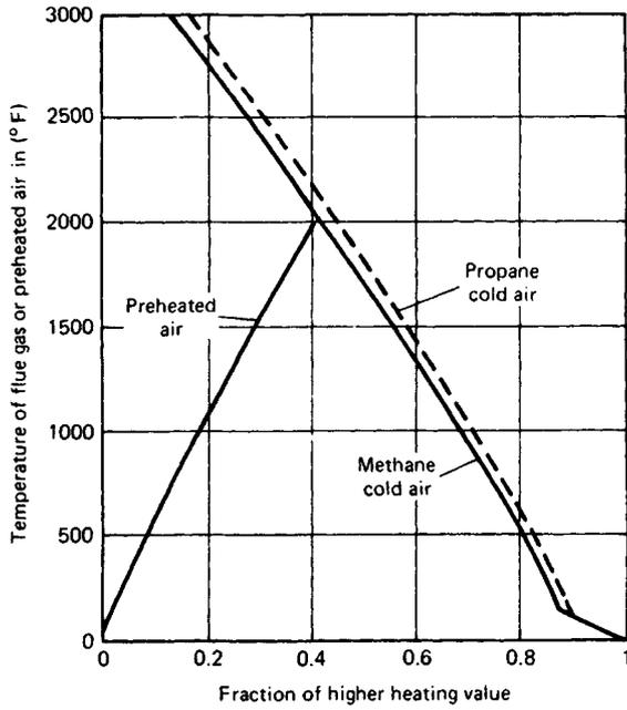
**Fig. 45.1** Available heat for methane and propane combustion. Approximate high and low limits for commercial natural gas.<sup>1</sup>
