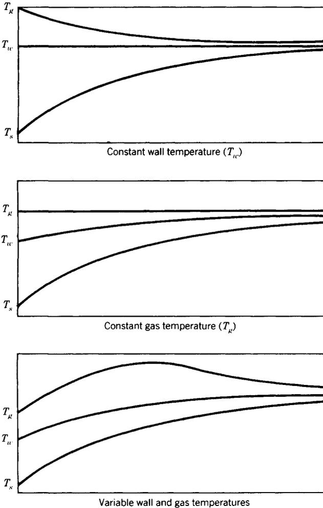
Fig. 45.27 Furnace temperature profiles.
