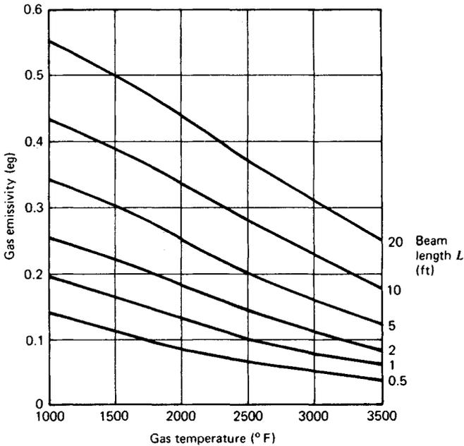
**Fig. 45.20** Gas-emissivity for products of combustion of methane burned with 110% air. Approximate for fuel oils and coke oven gas.<sup>1</sup>
