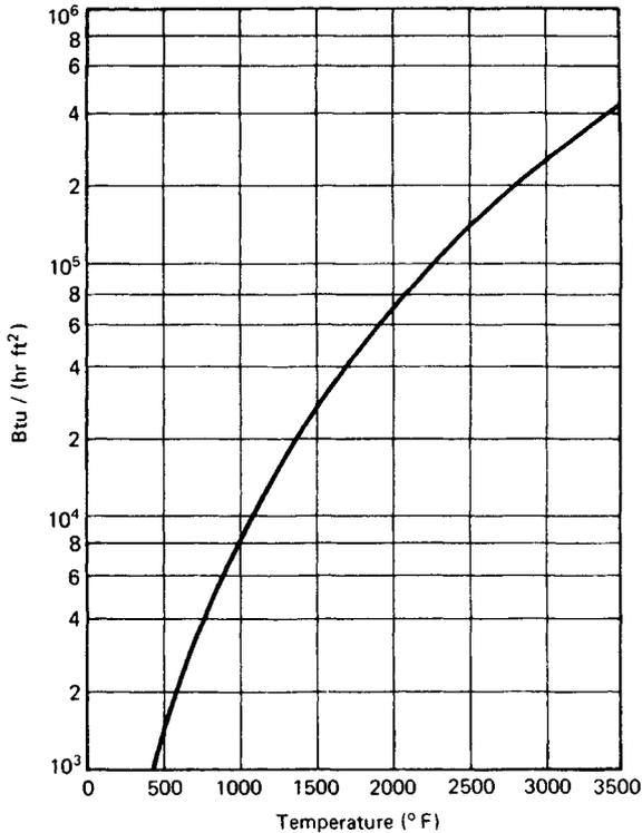
**Fig. 45.12** Black-body radiation as function of load surface temperature.
