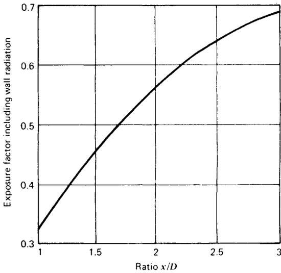
Fig. 45.17 View factors for spaced cylinders with back-up wall.<sup>1</sup>
