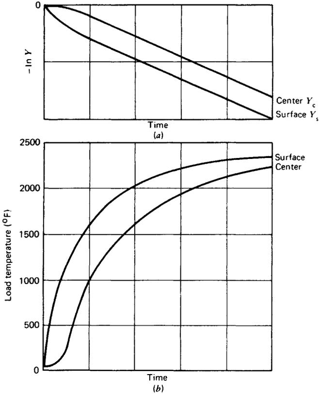
**Fig. 45.22** Maximum and minimum load temperatures, and  $-\ln Y_s$  or  $-\ln Y_c$  as a function of heating time with constant source temperature.<sup>1</sup>
