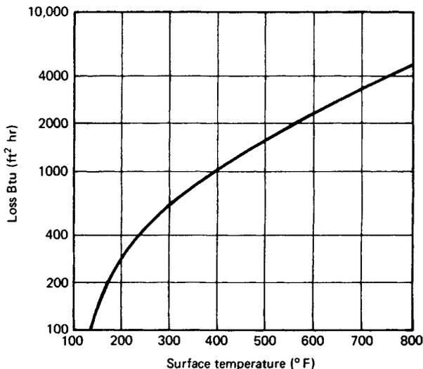
Fig. 45.7 Furnace wall losses as a function of surface temperature.<sup>1</sup>
