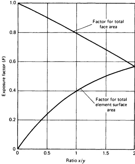
Fig. 45.18 View factors for ribbon-type electric heating elements mounted on back-up wall.<sup>1</sup>
