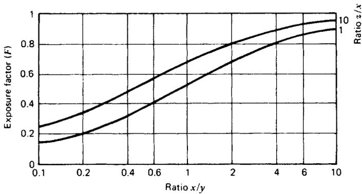
Fig. 45.19 View factors for parallel planes connected by reradiating sidewalls.<sup>1</sup>
