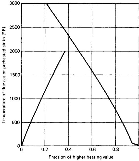
Fig. 45.3 Available heat ratios for by-product coke oven gas.<sup>1</sup>
