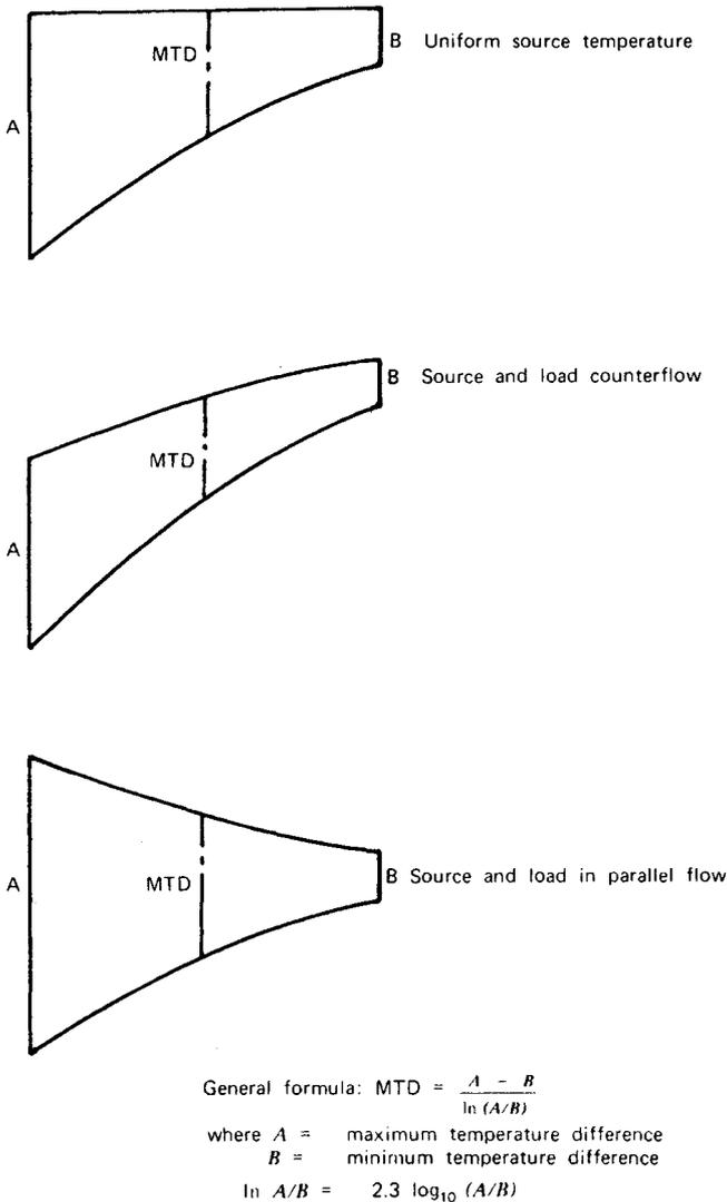
Fig. 45.10 Diagrams of log mean temperature difference (MTD).<sup>1</sup>
