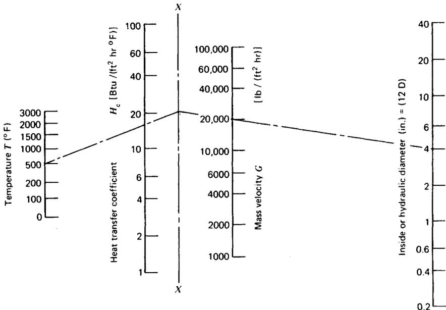
Fig. 45.28 Convection coefficient ( $H_c$ ) for forced convection inside tubes to air or flue gas.<sup>1</sup>
