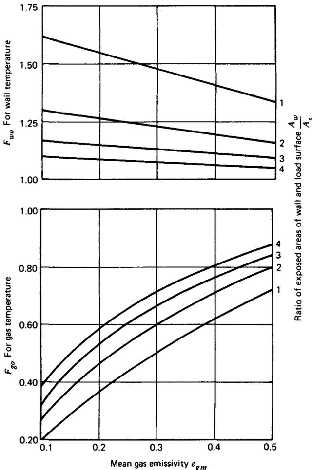
**Fig. 45.21** Overall heat-transfer coefficients for gas and solid radiation, as function of gas emissivity and wall-to-load area ratio, for uniform gas or wall temperature, compared to black-body radiation.<sup>1</sup>
