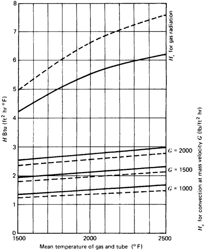
Fig. 45.31 Gas radiation ( $H_r$ ) and convection ( $H_c$ ) coefficients for flue gas inside radiant tubes.<sup>1</sup>
