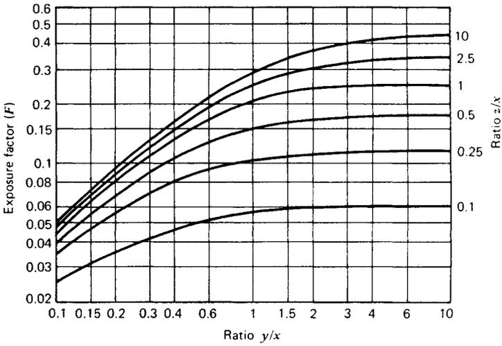
Fig. 45.16 Radiation view factors for perpendicular planes.<sup>1</sup>
