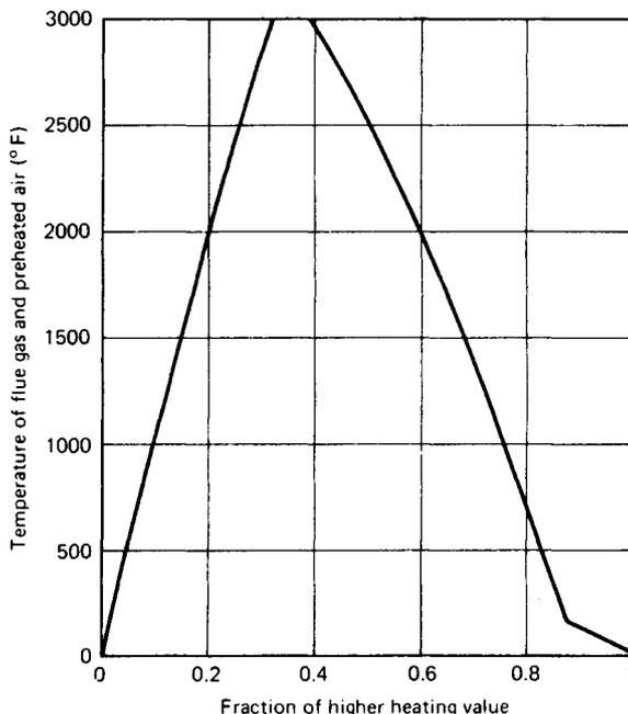
**Fig. 45.5** Available heat ratios for combustion of methane with 110% air containing 35% O<sub>2</sub>.<sup>1</sup>
